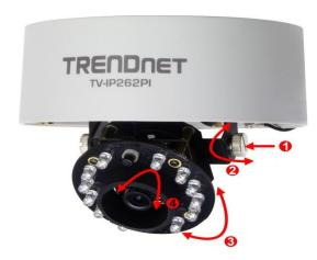
**NOTE:** You can review the image quality from the Web browser when you complete the installation. If the image quality is poor, you have to disassemble the Dome cover to adjust the lens focus until the desired image appears clearly.
